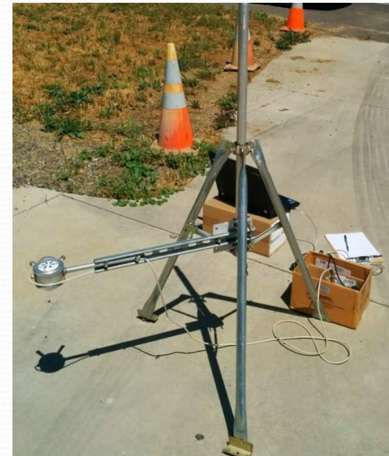
Albedometer with dual-pyranometer
