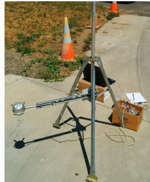
Albedometer with dual-pyranometer
